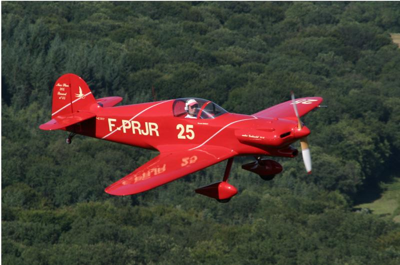
Built by Bernard Marichy between 1980 and 1995 on the Chambéry air force base, and then on the Toulouse-Francazal air force base, this Busard is powered by a Continental C-90-8F engine, of only 90hp. This aiplane is often seen at airshows in South-Western France. The addition of wheel fairings for the 2005 races has allowed an increase of the top speed of some 15 km/h.
