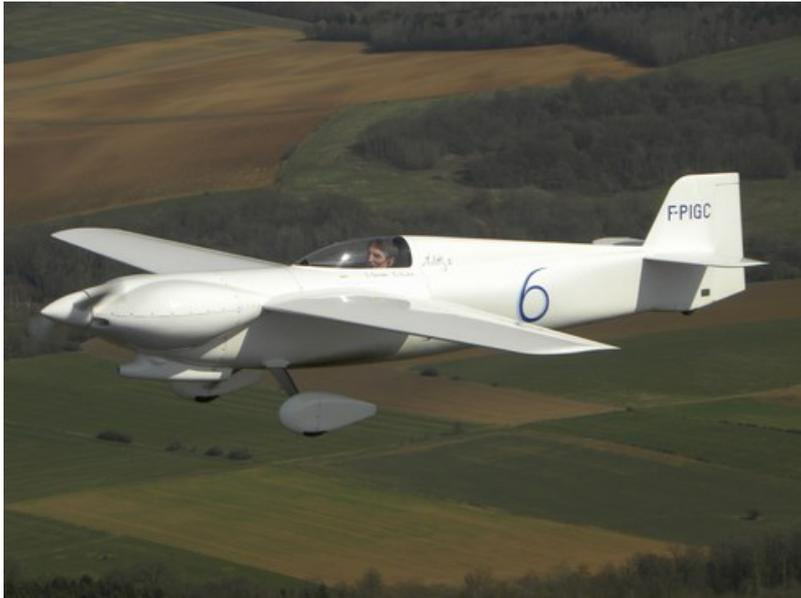
The Arletty II racer was completely designed and built by Christian Guilié between 2003 and 2009. The airplane is almost entirely built in composites, with only the wing spar made of wood. The fuselage is a monocoque sandwich structure (Airex foam/glass-epoxy). The wing, made of fiberglass as well, uses a laminar flow airfoil.
